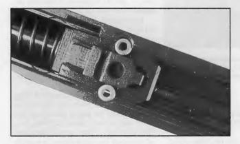
CZ Model 52's roller-locked breech system locks the barrel and slide together by means of two opposed vertical rollers held in recesses in the slide by the locking wedge, a sleeve-like piece that encircles the barrel ahead of the barrel lug.
